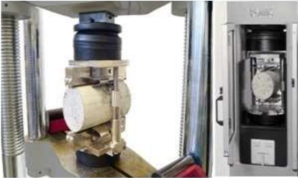
Fig.1: Split cylinder testing machine
